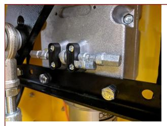
This image shows the gearbox disengaged
